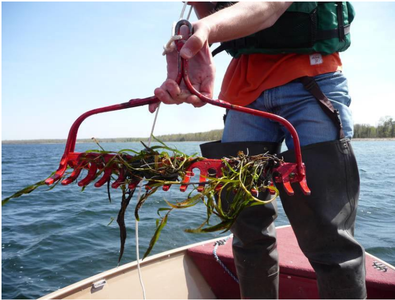
Figure 2. Double-headed, weighted garden rake, attached to a rope used to survey aquatic vegetation.
